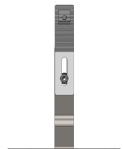
Tile Interface connection with elongated hole
